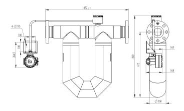
Fig.8 The overall dimensions of AMF080 model and order code for std.sensor: WS2LC-C1MD1-NGH08CPEN
