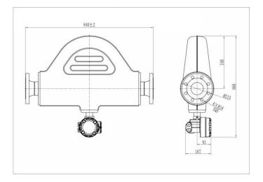
Fig.9 The overall dimensions of AMF080 model and order code for std.sensor:  ${\tt WS2NC-C1MD1-NGH05CPEN}$
