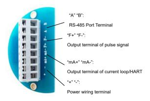
Fig.20 The layout diagram of the wiring of wring chamber of T2000 Transmitter
