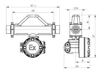
Fig.3 The overall dimensions of AMF015 model and order code for std.sensor: RS2NG-C1MD1-NGG01CPEN
