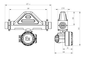
Fig.4 The overall dimensions of AMF020 model and order code for std.sensor:  ${\tt RS2NH-T1MD1-NGG02CPEN}$
