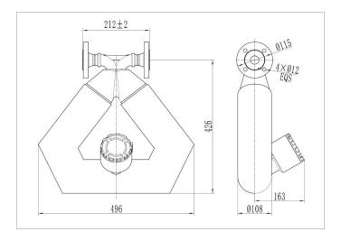
Fig.5 The overall dimensions of AMF025 model and order code for std.sensor: WS2LB-C1MD1-NSH02CPEN
