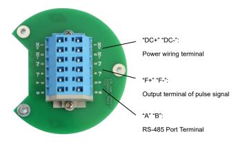
Fig.17 The layout diagram of the wiring of wring chamber of T1000 Transmitter
