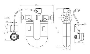
Fig.6 The overall dimensions of AMF050 model and order code for std.sensor: WS2LC-C1MD1-NGH04CPEN
