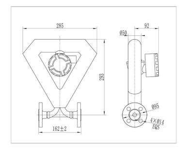
Fig.2 The overall dimensions of AMF008 model and order code for std.sensor:WS2LA-C1MD1-NSH01CPEN
