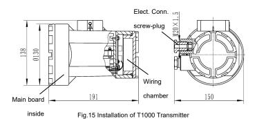
Threading hole of power wire
