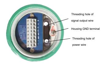
Fig.19 The layout diagram of the wiring chamber of T2000 Transmitter
