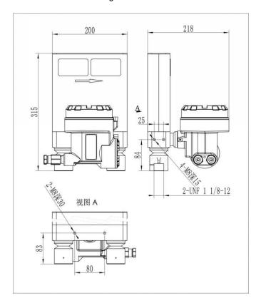
Fig.1 The overall dimensions of AMF006 model and order code for std.sensor:QS1NA-C3MD1-NGP02DPFN
