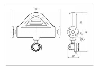
Fig.7 The overall dimensions of AMF050 model and order code for std.sensor:
